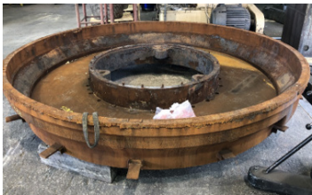
Ceramic Liner on Roll Wheel Bracket – Original OEM design did not supply any wear resistant material or line the cast
