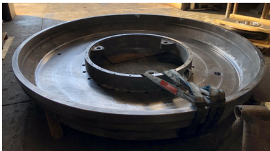
Ceramic Liner on Roll Wheel Bracket – Original OEM design did not supply any wear resistant material or line the cast
