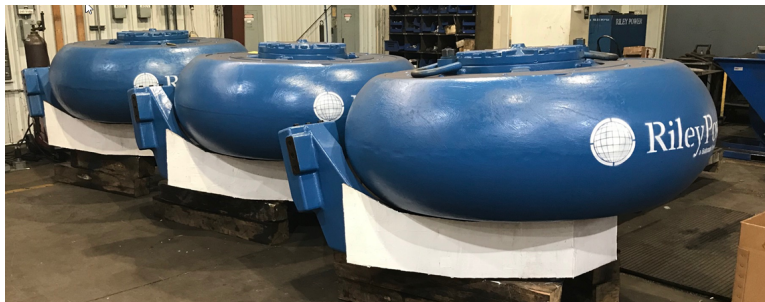
Ceramic Liner on Roll Wheel Bracket – Original OEM design did not supply any wear resistant material or line the cast
