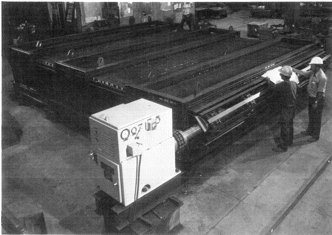
Figure 17 Shop Assembled, Modular Riley Traveling Grate
