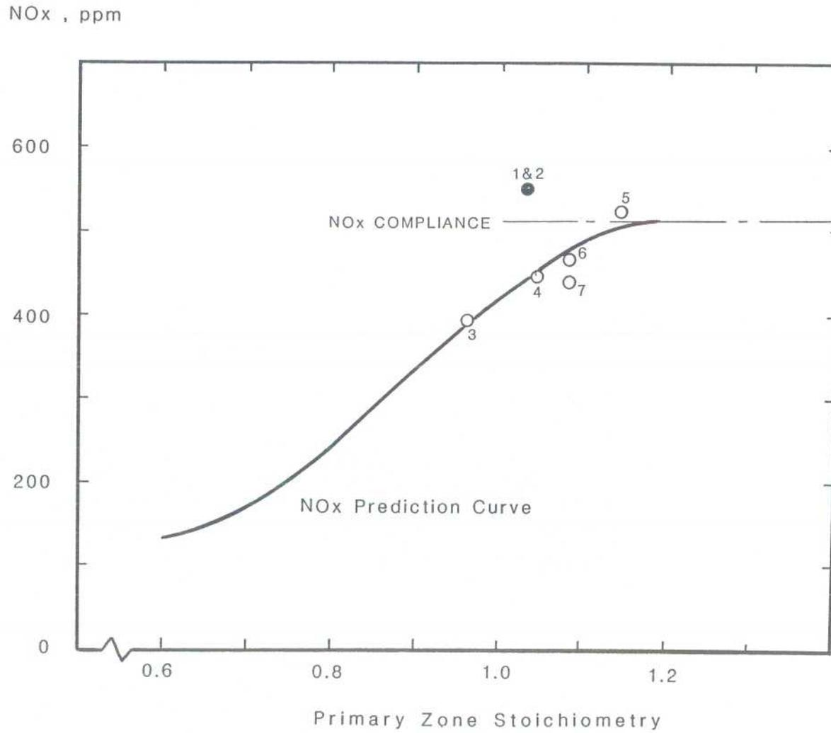
Figure 2. CCV Burner Performance at a 360 MWe Unit
