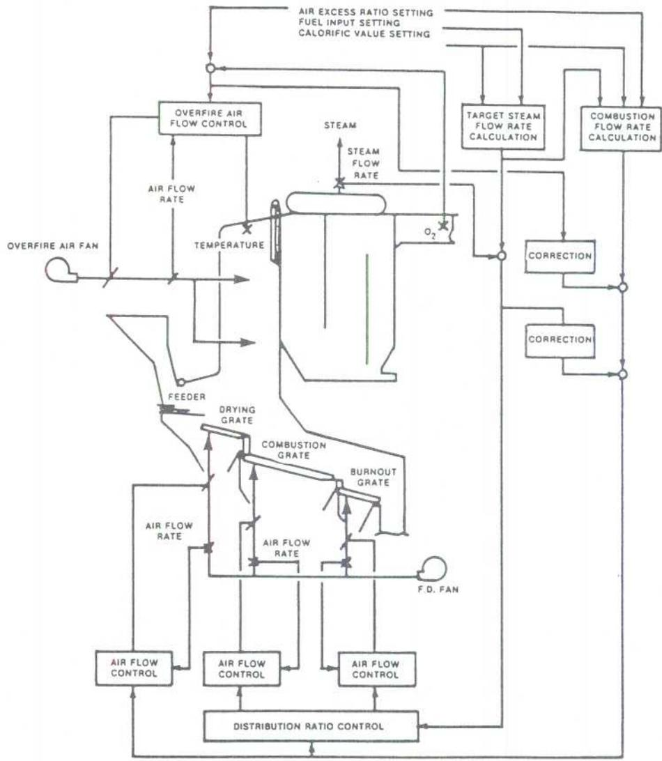
Figure 7b. Schematic Diagram of Riley/Takuma Combustion Air and Low Oxygen Control System
