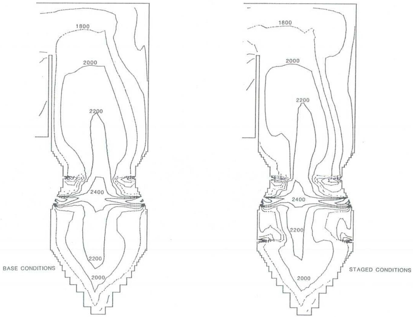
Figure 5. Temperatures for Original and Staged Operating Conditions
