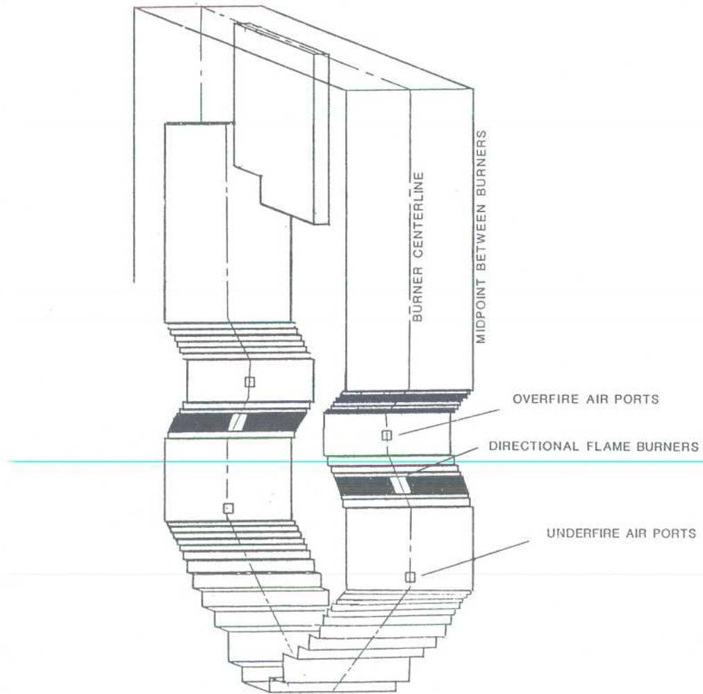
Figure 4. Isometric View of Furnace Modeling Domain
