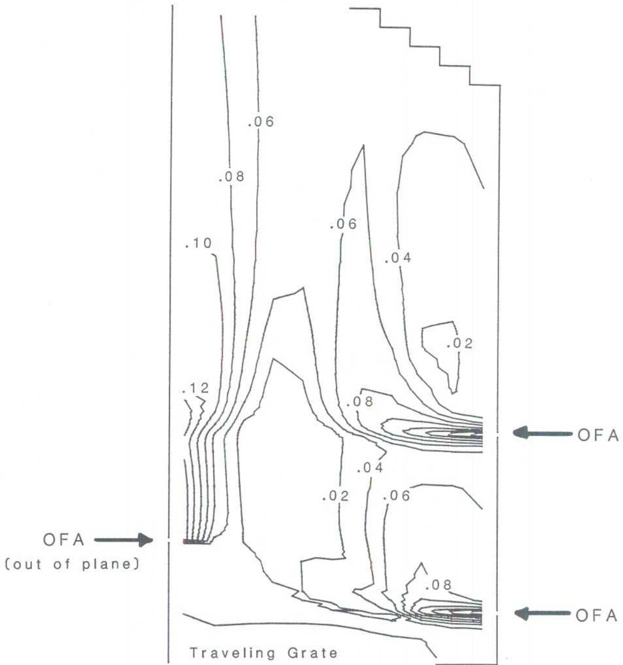
Figure 6. Predicted Oxygen Mass Concentration Profiles for an RDF-Fired Boiler with Multiple Levels of Overfire Air Injection
