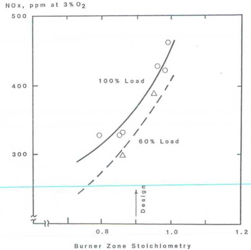
Figure 3b. NO<sub>x</sub> vs. Burner Zone Stoichiometry for the TSV System (Coal Firing at 100% and 60% Load)
