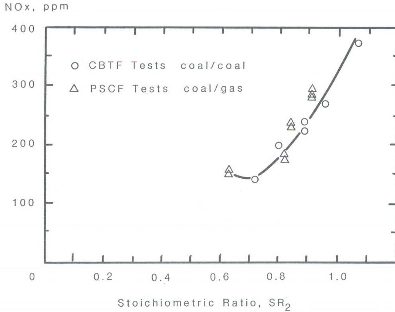
Figure 12. Reburning Test Results -  $100 \times 10^6$  Btu/hr CBTF and  $3 \times 10^6$  Btu/hr PSCF
