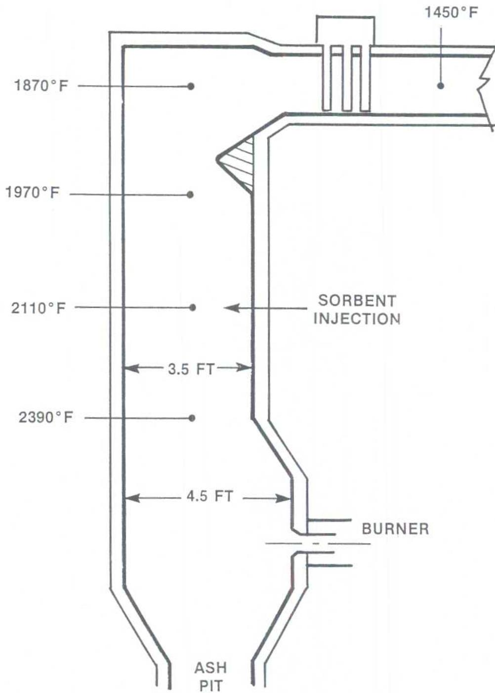
Figure 10.  $3 \times 10^6$  Btu/hr. Pilot-Scale Combustion Facility
