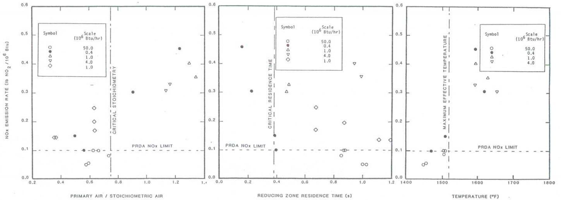
Figure 9. NOx Emissions Data from MSFBC Systems
