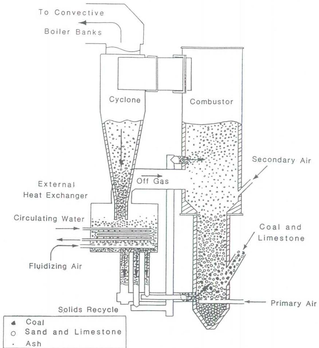
Figure 8. Multi-Solid Fluidized Bed Combustion Process
