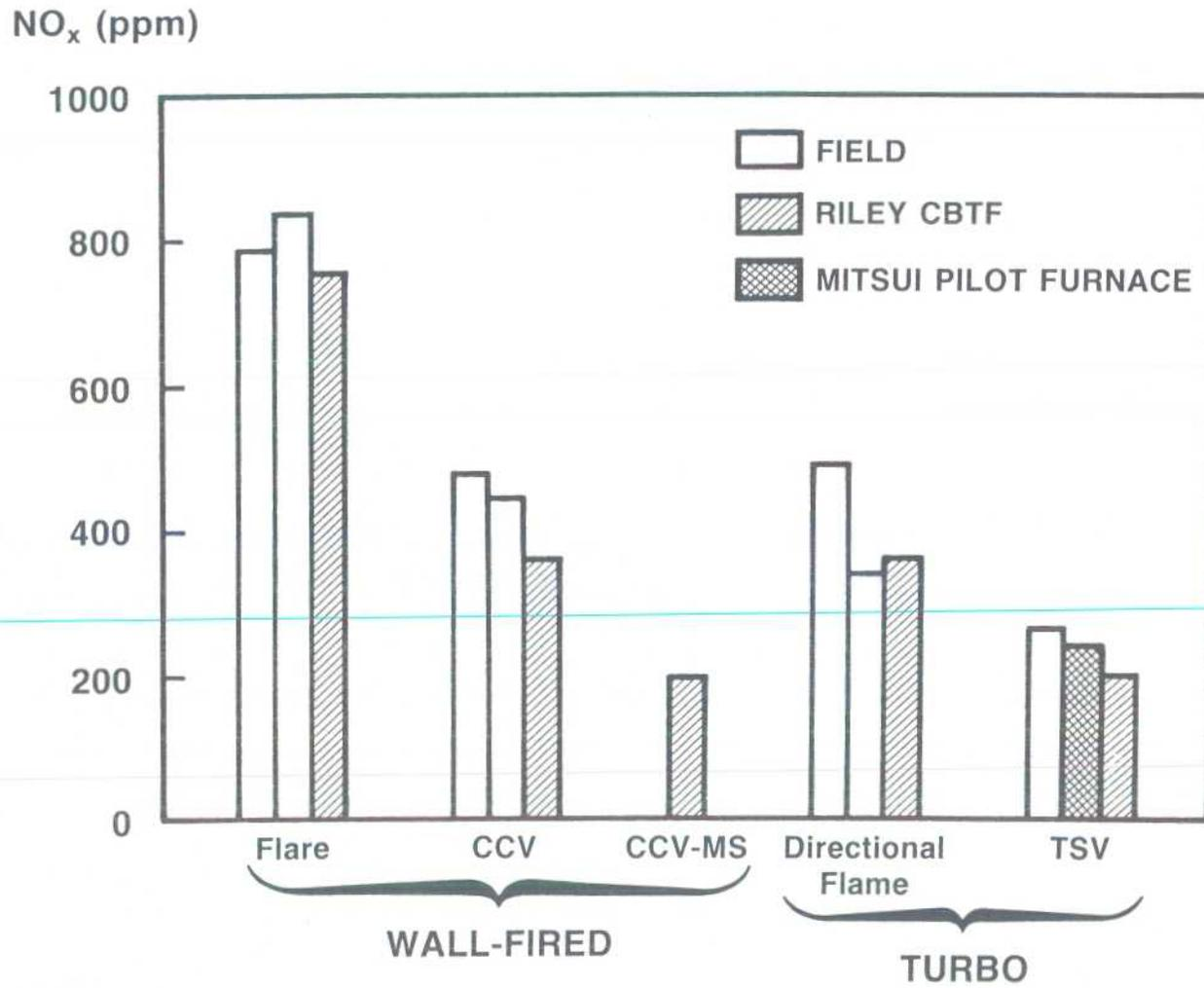
Figure 1. Burner Performance Comparison
