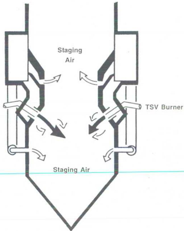
Figure 3a. Advanced Turbo Furnace Staging System
