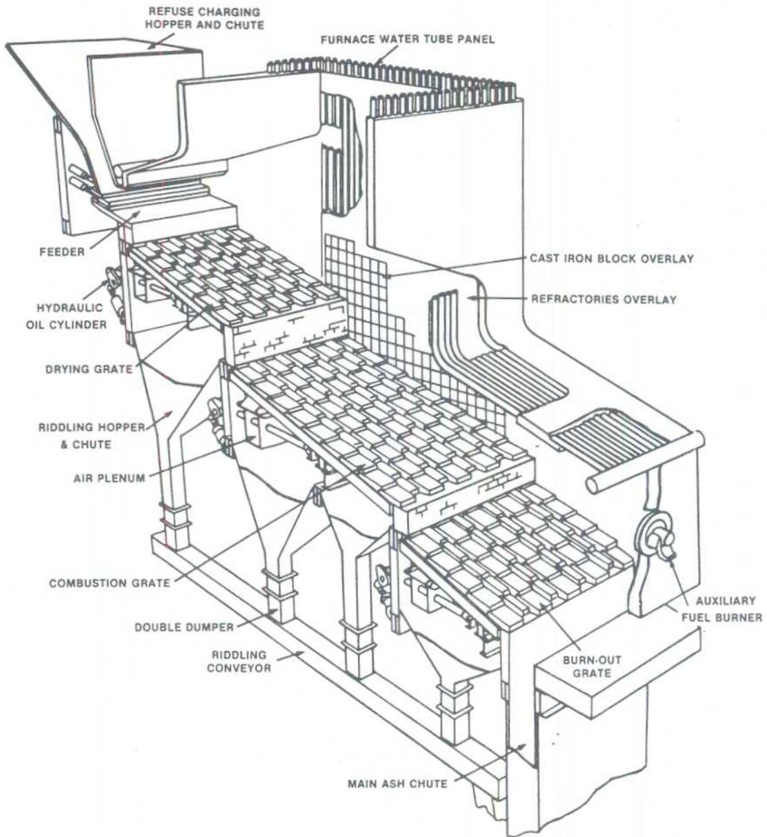
Figure 7a. Riley/Takuma Municipal Solid Waste Combustion System
