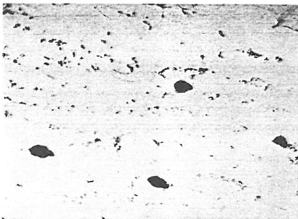
Figure 1.3 Microstructure At The OD Of The Tube. Large Black Spots Are Graphite. Nital Etch, 500x.
