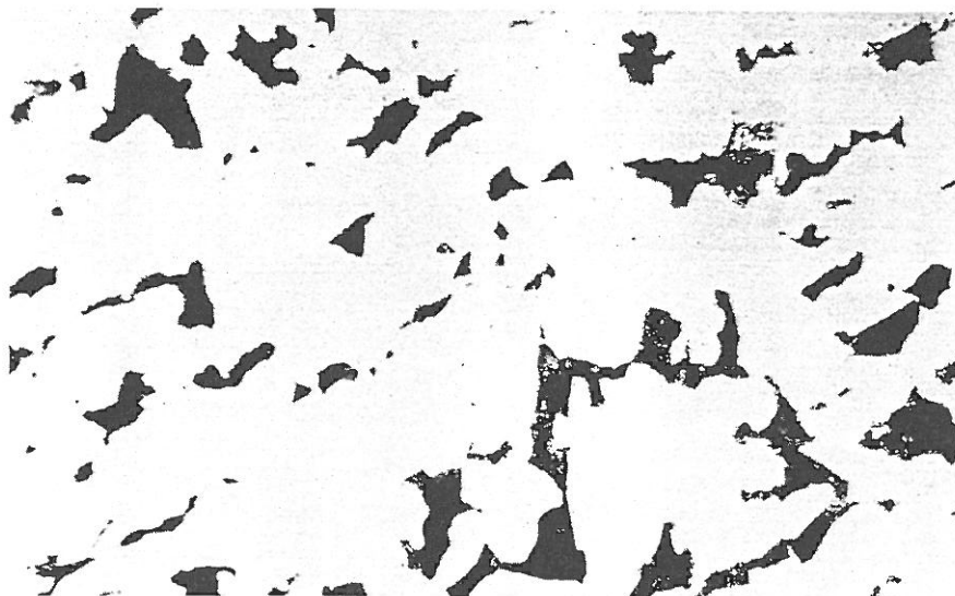
Figure 1.5 Microstructure Of The Back Side Of The Tube. The Structure Is Pearlite (Dark Areas), And Ferrite (Light Areas), And Is The Normal, Expected Structure For SA 210 A1. Nital Etch, 500x.
