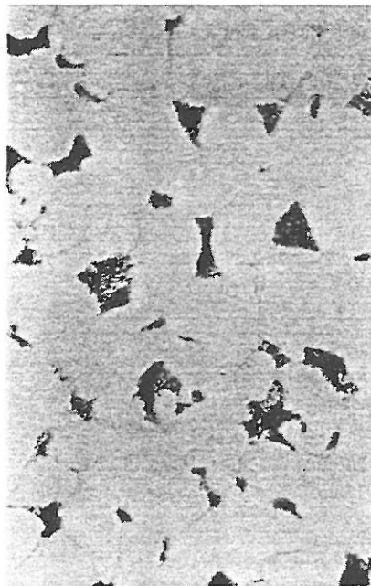
Figure 3.4 The Microstructure Of The Same Tube Taken From The Rear Of The Tube, 180° From The Rupture, The Structure Is Pearlite With An In Situ Spheroidization Of The Carbide Phase, And Ferrite. Nital Etch, 500x.
