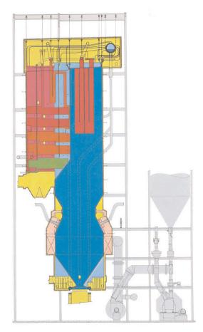
Figure 3. General Arrangement of Steam Generator being converted from Bituminous to PRB Coal
