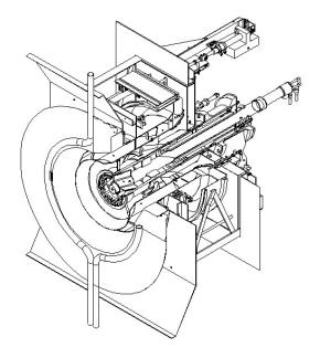
Figure 2.  $CCV^{\mathbb{R}}$  DAZ Low  $NO_X$  burner installation
