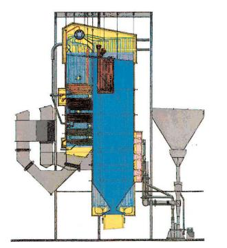
Figure 1. General Arrangement of Steam Generator being converted from Bituminous to PRB Coal
