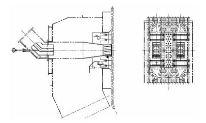
Figure 4. Upgraded Directional Flame Burner with Fixed position Low NO<sub>x</sub> Coal Nozzles
