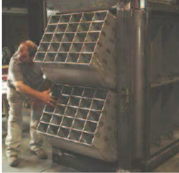
Figure 3. Comanche 1 Separated OFA Windbox Assembly
