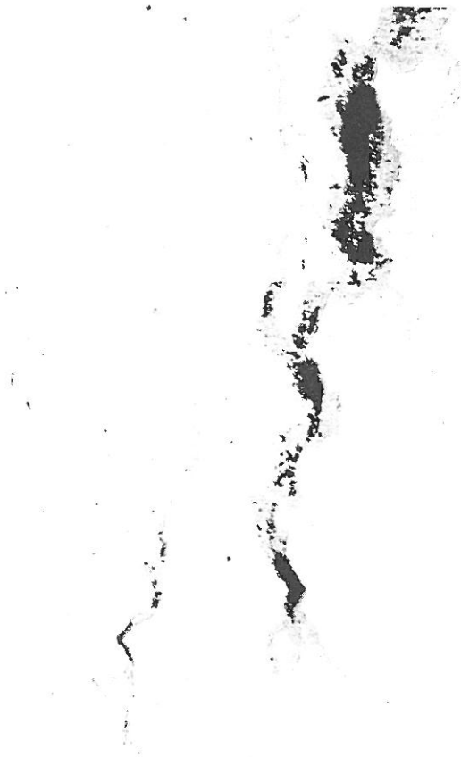
Figure 9. Photomicrograph from the Figure 8 specimen of a longitudinal, intergranular crack (100×)
