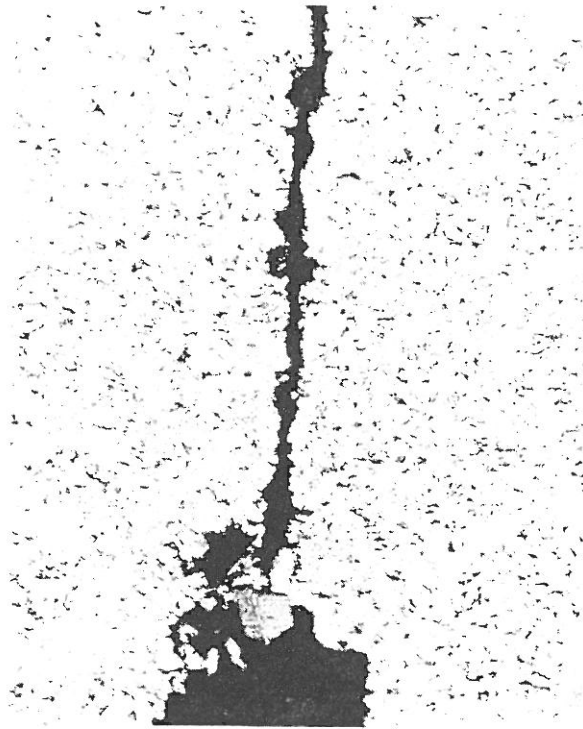
Figure 3. Photomicrograph of a crack from the Figure 2 sample, originating at a corrosion filled internal pit (100X)
