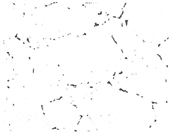
Figure 10. Enlargement of the structure from the Figure 9 photomicrograph, showing creep voids at grain boundary triple points (500×)
