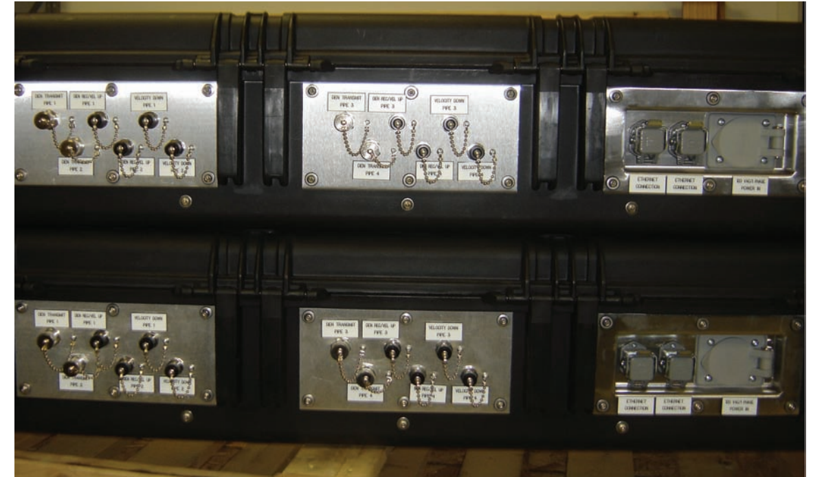
Figure 1 — Riley Portable Pf-FLO III Reads up to 8 coal pipes simultaneously
