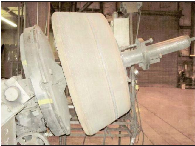
Figure 2: Photograph of roll with Clad-Tech process
