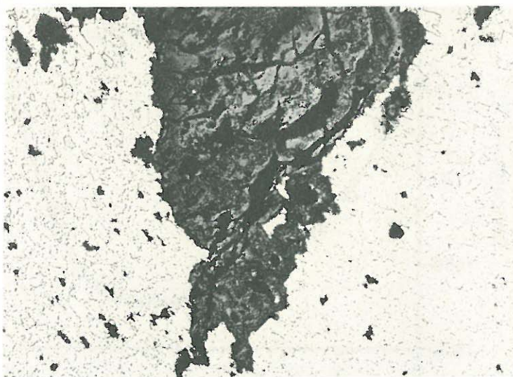
Figure 11 The Structure at or near the Tip of the Failure. Note that the Crack is Completely Filled with Oxide Scale. The Black Specks in the Metal are Voids Indicative of a Creep Failure. (500X, Nital Etch)
