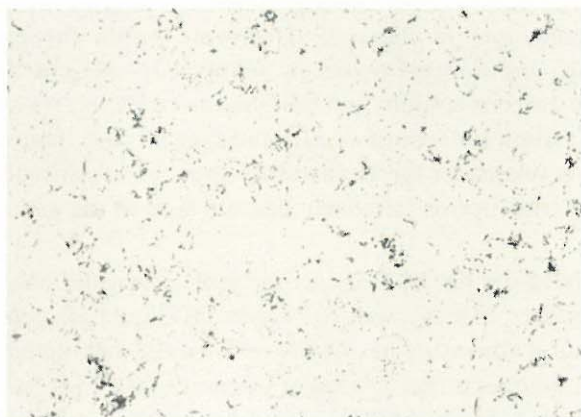
Figure 9 Microstructure Shows Spheroidized Carbides and Ferrite (500X, Nital Etch)
