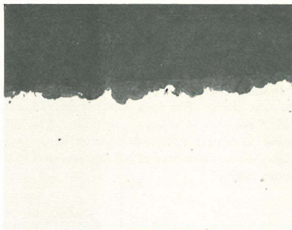
Figure 24 Interface Morphology of Steam Side Oxide on SA 213-TP321 Tubing. Note the Unevenness to the Scale/Metal Interface. (70X, Unetched)
