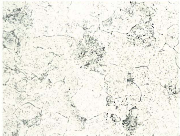
Figure 18 Microstructure of As-received New T-22 Tubing. Compare the Changes in Carbide Morphology. (350X, Nital Etch)
