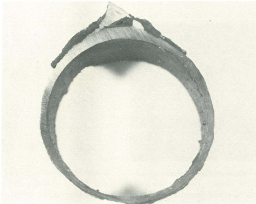
Figure 20 Cross-sectional View of an As-received T-22 Reheater Tube. Note the Extensive Metal Wastage in the Lower Portion of the Photograph.
