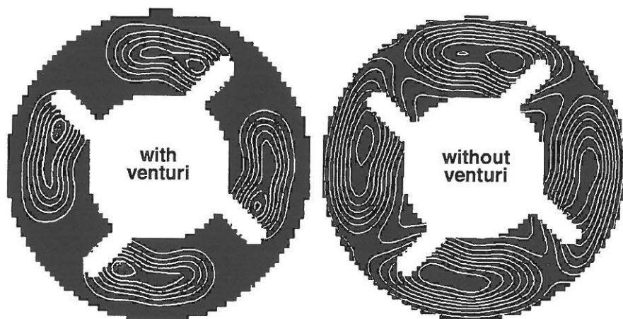
Figure 3 Particle mass density in the coal nozzle for a CCV® burner. (Reaction Engineering International)
