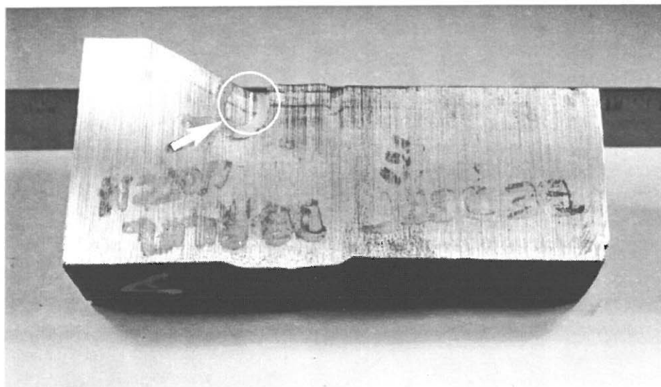
Figure 1 The cut cross-sectioned surface of the sample weldment, showing the location of a circumferential crack at the taper transition at the inside of the elbow to pipe junction.
