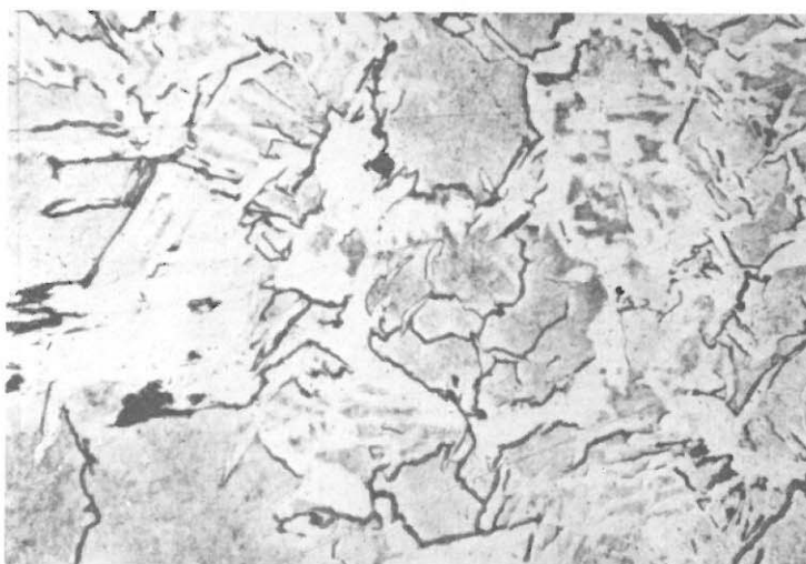
Figure 3 Hydrogen Damage Manifested as Cracks in Weld — Case Study No. 2 (500X)
