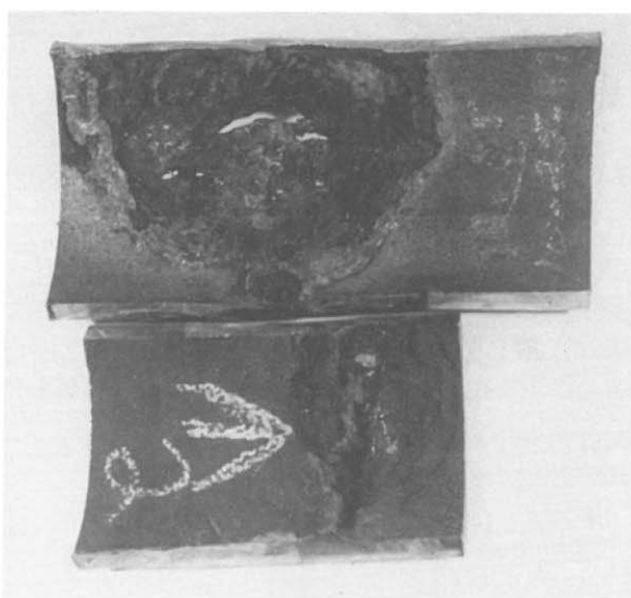
Figure 2 I.D. of As-Received Failed Tubes — Case Study No. 2 Note the Localized Deposits and Gouging at Welds
