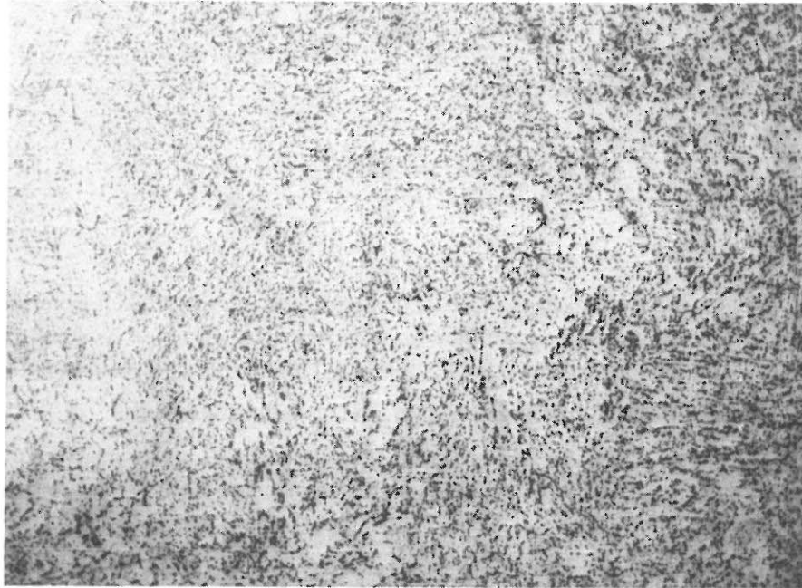
Figure 2.2 Microstructure of As-received T-22 Tubes; the Carbides are Completely Spheroidized. (500 \times , Nital Etch)
