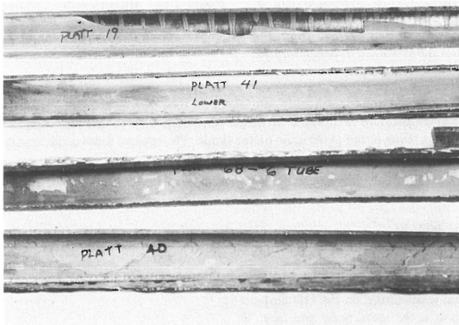
Figure 1.2 As-received Reheater Tubes. Note the Heavy Internal Oxide Scale.
