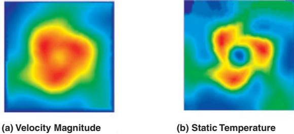
Figure 5. Typical Gas Turbine Velocity and Temperature Profiles Applied at the CFD Model Inlet
