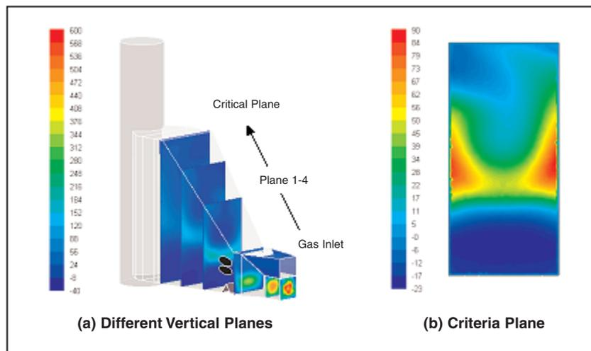
Figure 9. Calculated Axial Velocity Distributions (ft/s) for Case I
