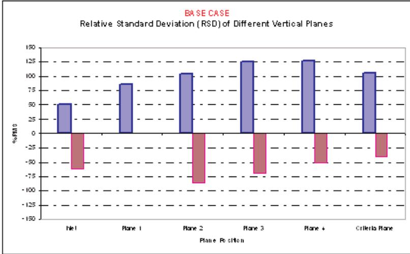
Figure 7. Calculated RSD (% rms) through Vertical Planes for the Base Case
