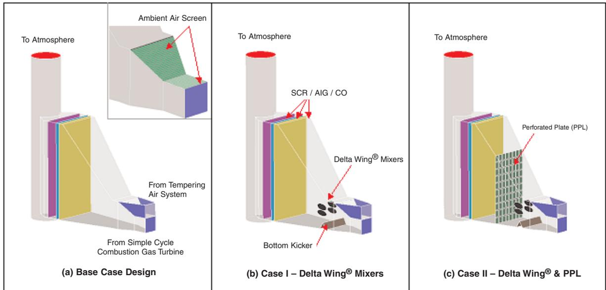
Figure 4. Schematic of the Three (3) Representative Simple Cycle SCR Configurations
