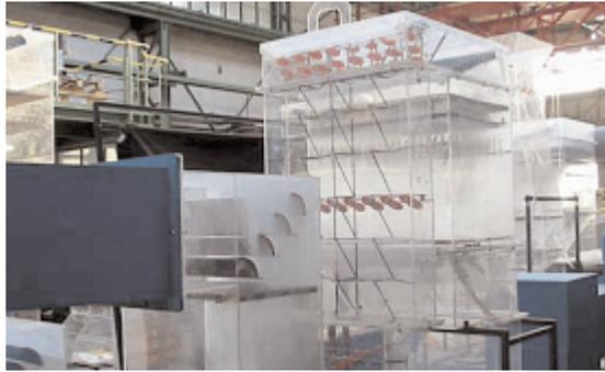
Figure 1. Installed Delta Wing® in a typical SCR Physical Flow Model
