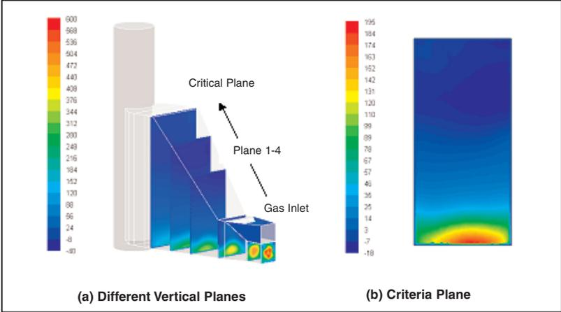
Figure 6. Calculated Axial Velocity Distributions (ft/s) for the Base Case
