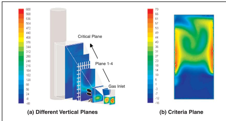
Figure 12. Calculated Axial Velocity Distributions (ft/s) for the Case II
