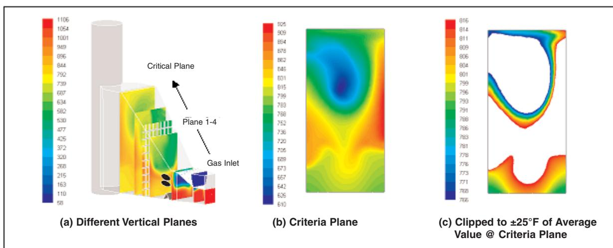
Figure 14. Calculated Temperature Distributions ( $^\circ\text{F}$ ) for the Case II
