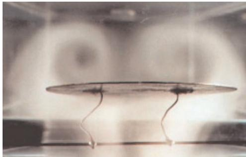
Figure 2. Illustration of the formation of Delta Wing® vortices
