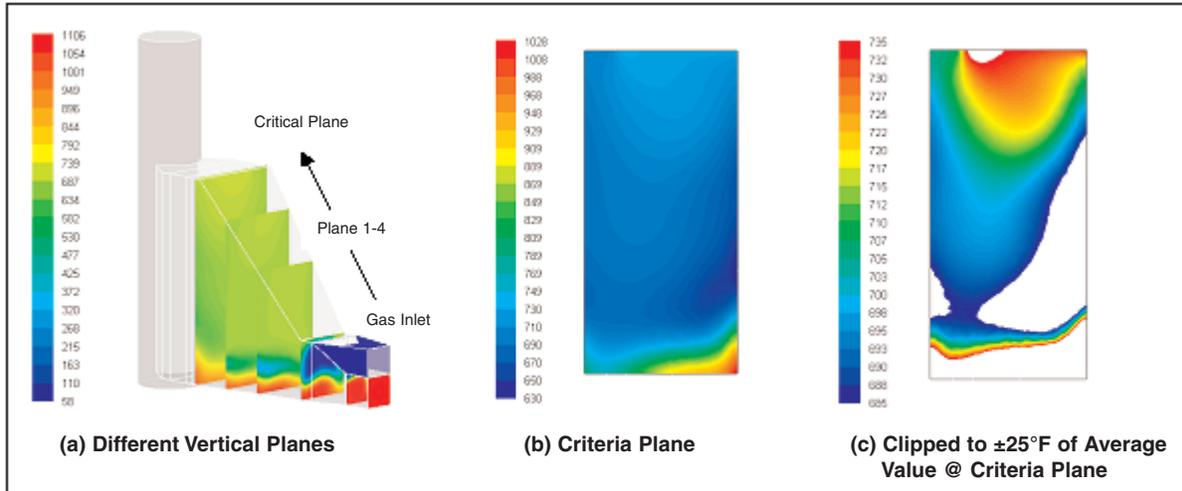
Figure 8. Calculated Temperature Distributions ( $^{\circ}\text{F}$ ) for the Base Case
