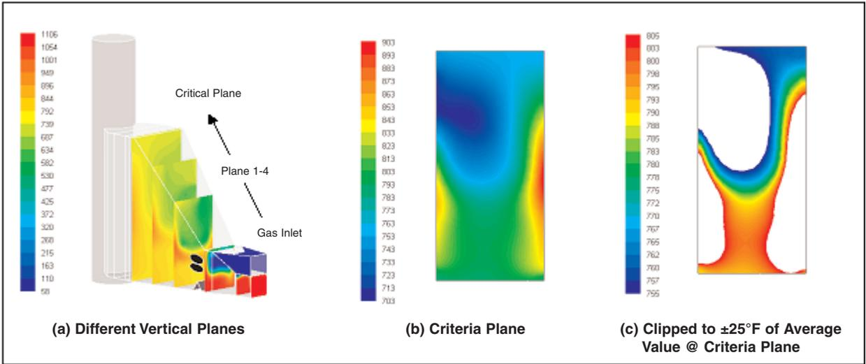
Figure 11. Calculated Temperature Distributions ( $^\circ\text{F}$ ) for Case I
