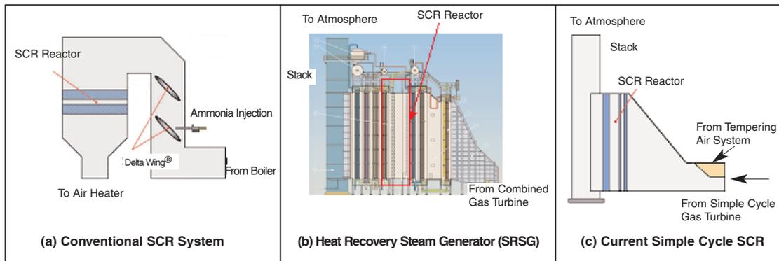
*Figure 3. Schematic Illustration of Different Selective Catalytic Reduction (SCR) Systems*
