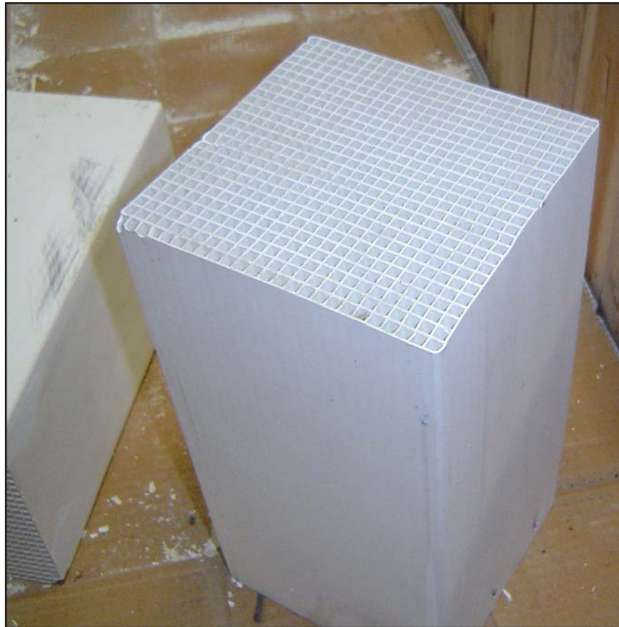
Figure 6. A block of monolith ceramic thermal media.
