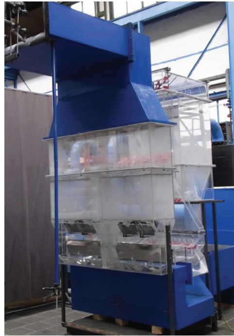
Figure 2 – TVA Gallatin SCR Dust Model (1:18 Scale)
