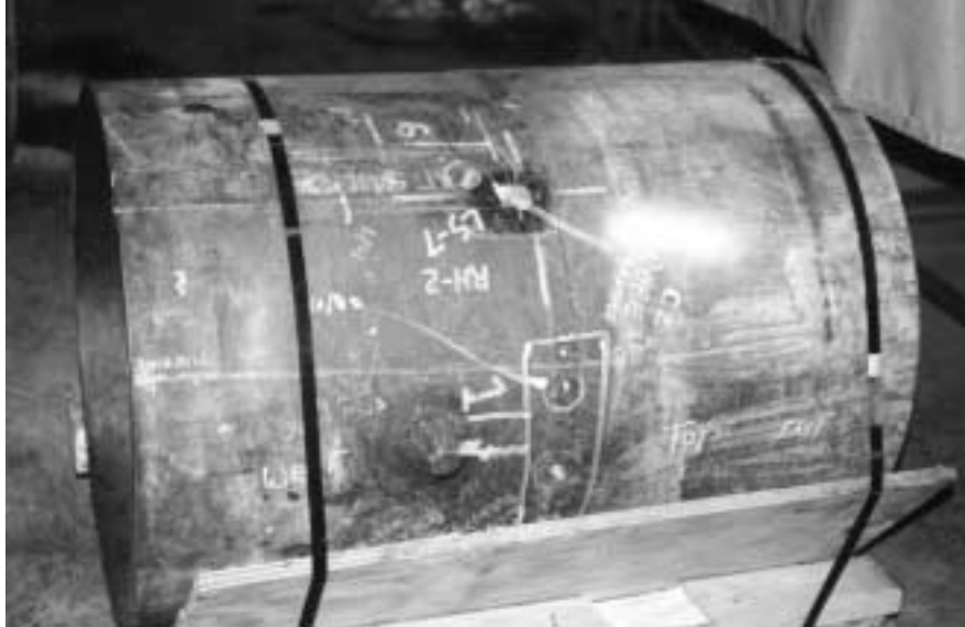
Figure 11 Hot reheat piping spool piece removed for testing and analysis.
