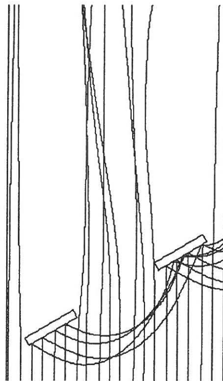
Figure 7 Coal Particle Trajectories. Coal particle diameter of 290 Microns, original blade design, attack angle 30^\circ , 20 particles injected.
