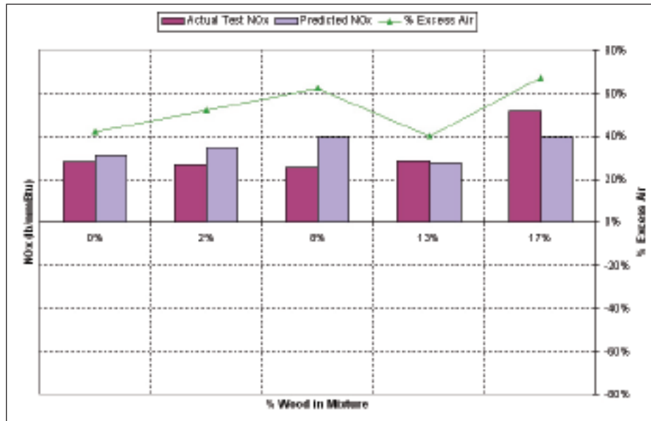
Figure 8. Comparison of NO x Prediction Versus Actual Measured NO x
