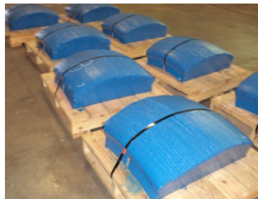
Pfeiffer MPS Tire Segments after overlay and carbiding
