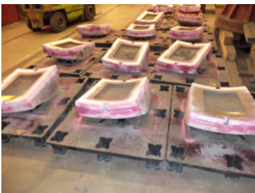
Worn Pfeiffer MPS Tire Segments before overlay and carbiding
