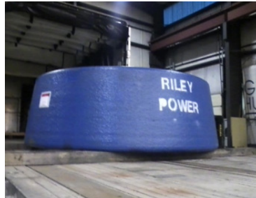
Loesche Grinding Roll after overlay and carbiding
