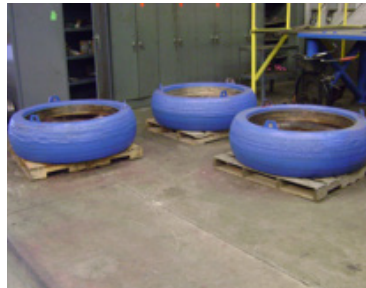
Polysius Doral Tire after overlay and carbiding
