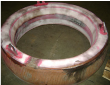
Worn Polysius Doral Tire before overlay and carbiding
