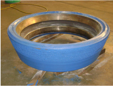
FLSmith Grinding Roll after overlay and carbiding
