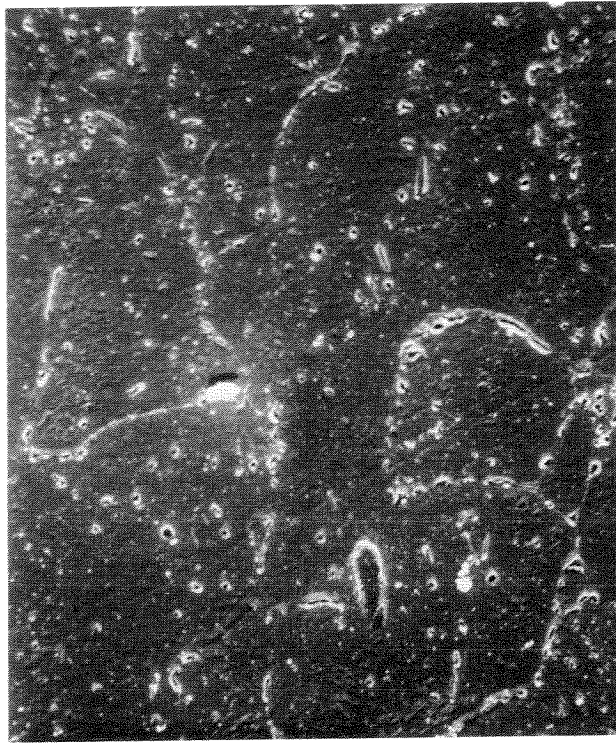
Figure 7 Scanning Electron Photomicrograph (1000X) of same replica showing evidence of isolated creep of microvoids which appear as bright spots. - Courtesy of Teledyne Engineering Services.
