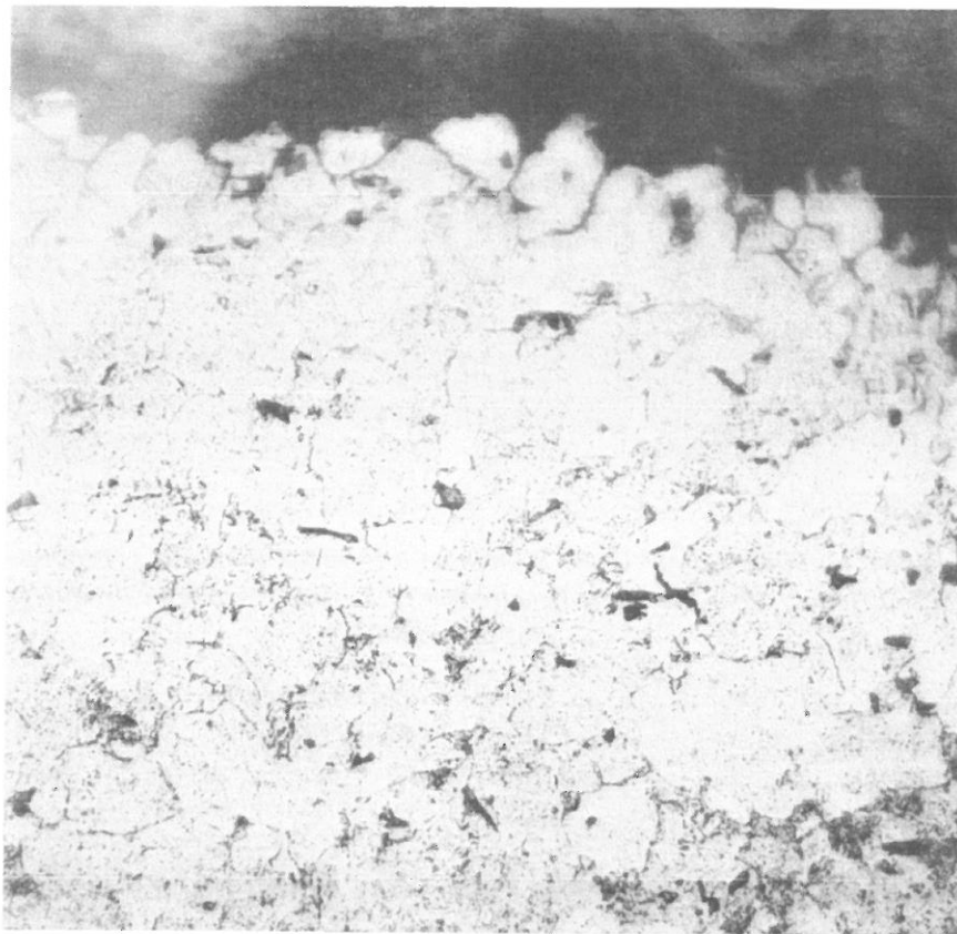
Figure 2 Microstructure of the Superheater Tube From Figure 1, Note the Intergranular Penetration of the Sulfide Corrosion Product. 250X
