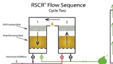
Figure 2: RSCR flow sequence – cycle two
