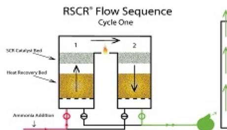
Figure 1: Operation of a two-canister RSCR design.
