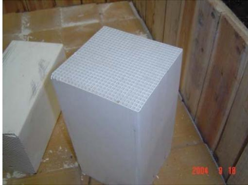
Figure 3: A block of monolith ceramic thermal media
