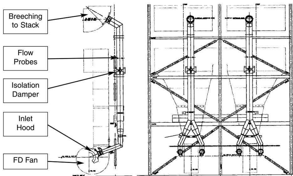
Figure 7 IFGR System Applied to Unit B
