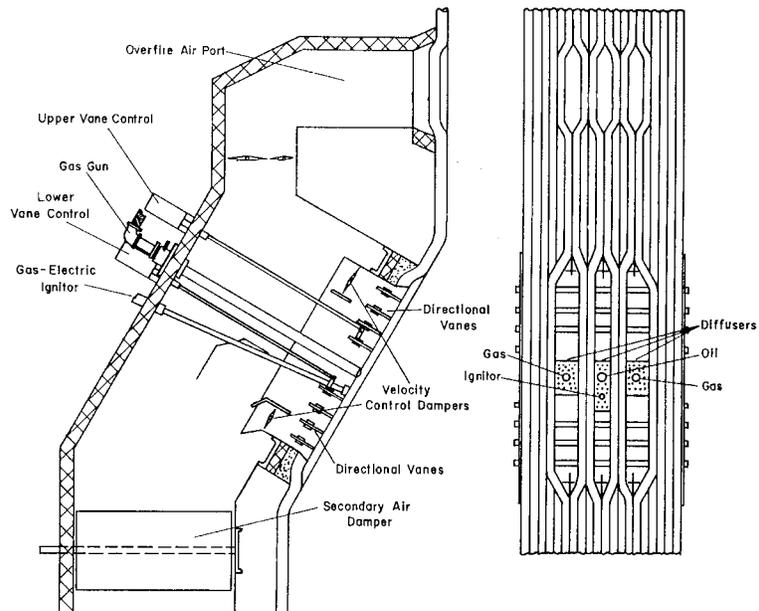
Figure 3 Unit A Original OFA Configuration
