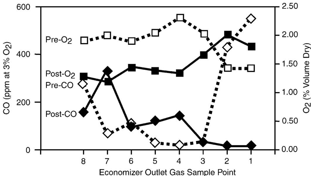
Figure 5 Comparison of Pre- and Post-retrofit Economizer Outlet CO and O<sub>2</sub> Profiles
