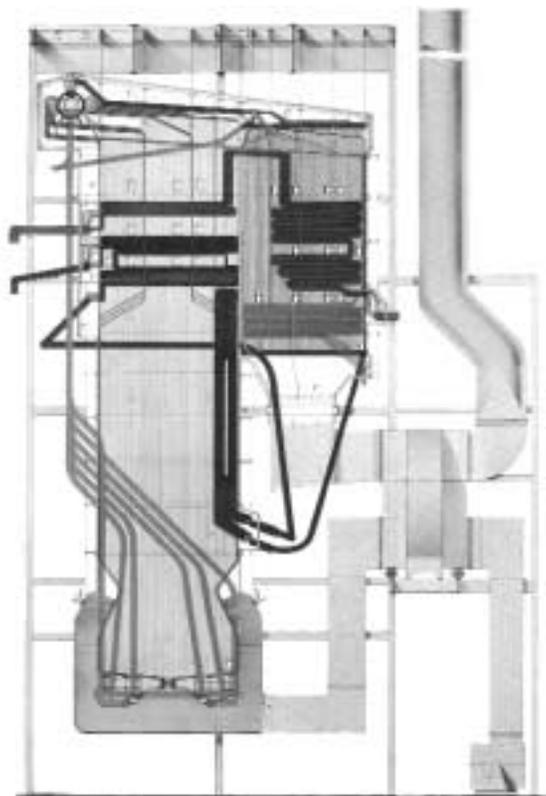
*Figure 6 Unit B Boiler Schematic*
