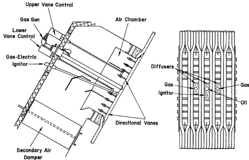
Figure 1 Typical Directional Flame Burner for Gas and Oil Firing
