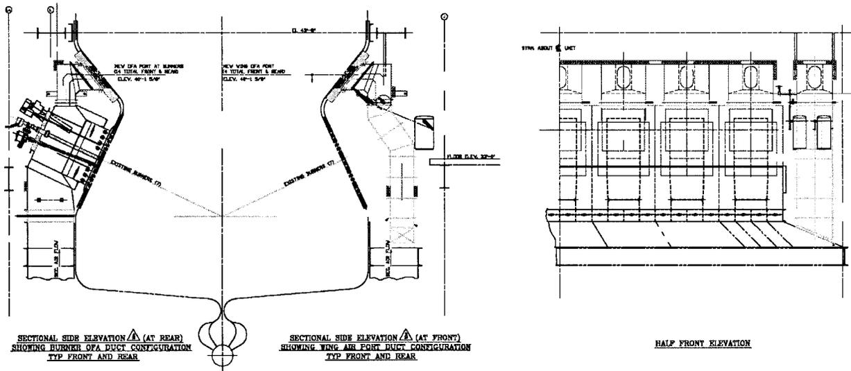
Figure 4 Windbox Partitioning Applied to Unit A
