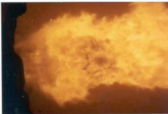
Figure 4 VS III™ Low NOx Burner Flame in Combustion Test Furnace
