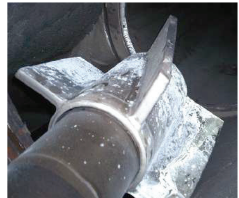
Figure 8 Coal Spreader with Conforma Clad® coating after 2 years of operation (highly abrasive Bituminous/pet coke blend)
