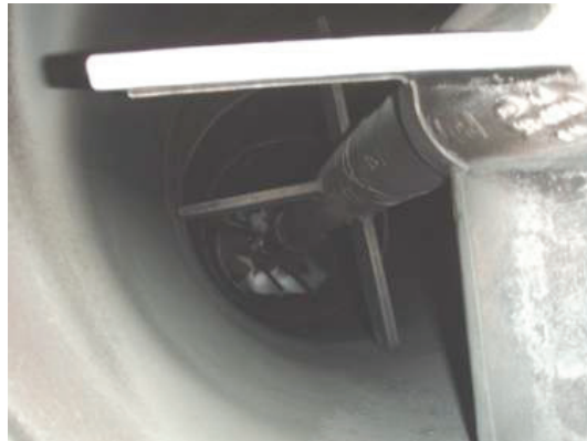
Figure 7 210 mmBtu/hr capacity burner on Foster Wheeler unit after 2 ½ years of operation (medium abrasive Galatia Bituminous coal)
