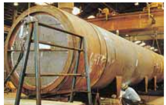
Preparation for final shell-to-skirt closing seam at our Joplin, MO facility
