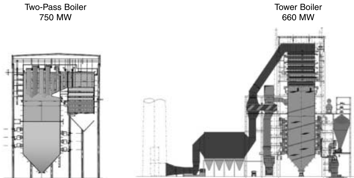
Figure 9 Examples of Once-through Boilers
