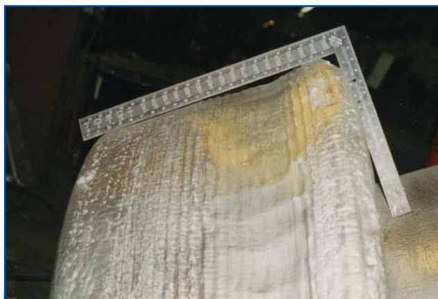
TUNGSTEN CARBIDE OVERLAY MINIMIZES WEAR EVEN AFTER 2,000,000 TONS OF LIGNITE.
