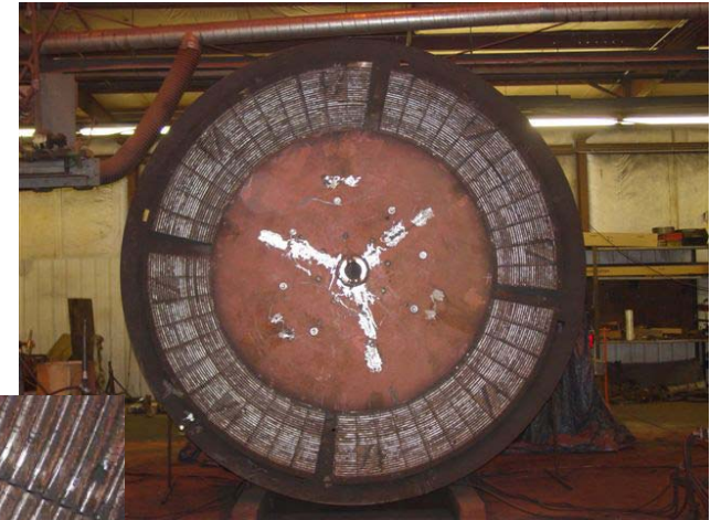
Bull Ring Segments grooved and ready for application of Clad-Tech™ C300TC Tungsten Carbide Matrix weld overlay.
